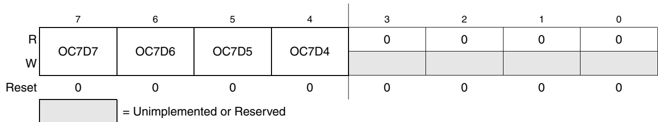
Figure 13-9. Output Compare 7 Data Register (OC7D)
