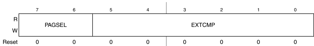
Figure 16-19. Debug Comparator B Extended Register (DBGCBX)
