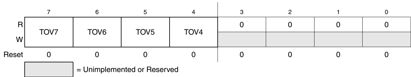
Figure 13-13. Timer Toggle On Overflow Register 1 (TTOV)
