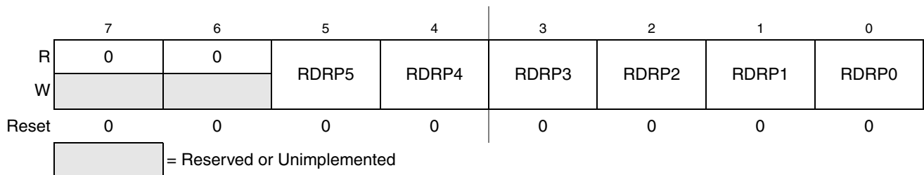
Figure 3-20. Port P Reduced Drive Register (RDRP)
