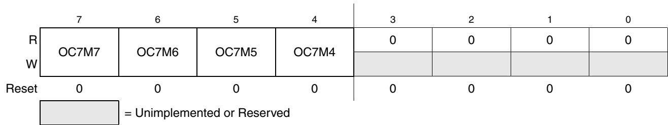
Figure 13-8. Output Compare 7 Mask Register (OC7M)
