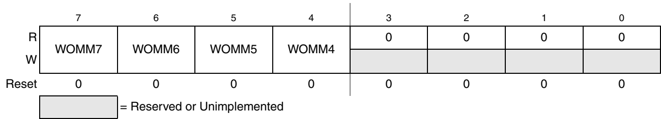
Figure 3-16. Port M Wired-OR Mode Register (WOMM)
