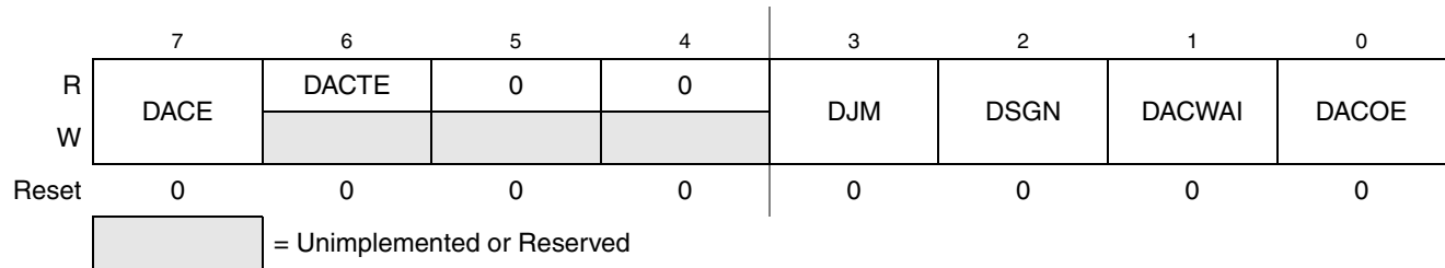
Figure 7-3. DAC Control Register 0 (DACC0)
