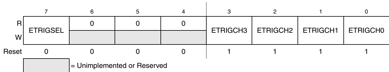
Figure 6-4. ATD Control Register 1 (ATDCTL1)
